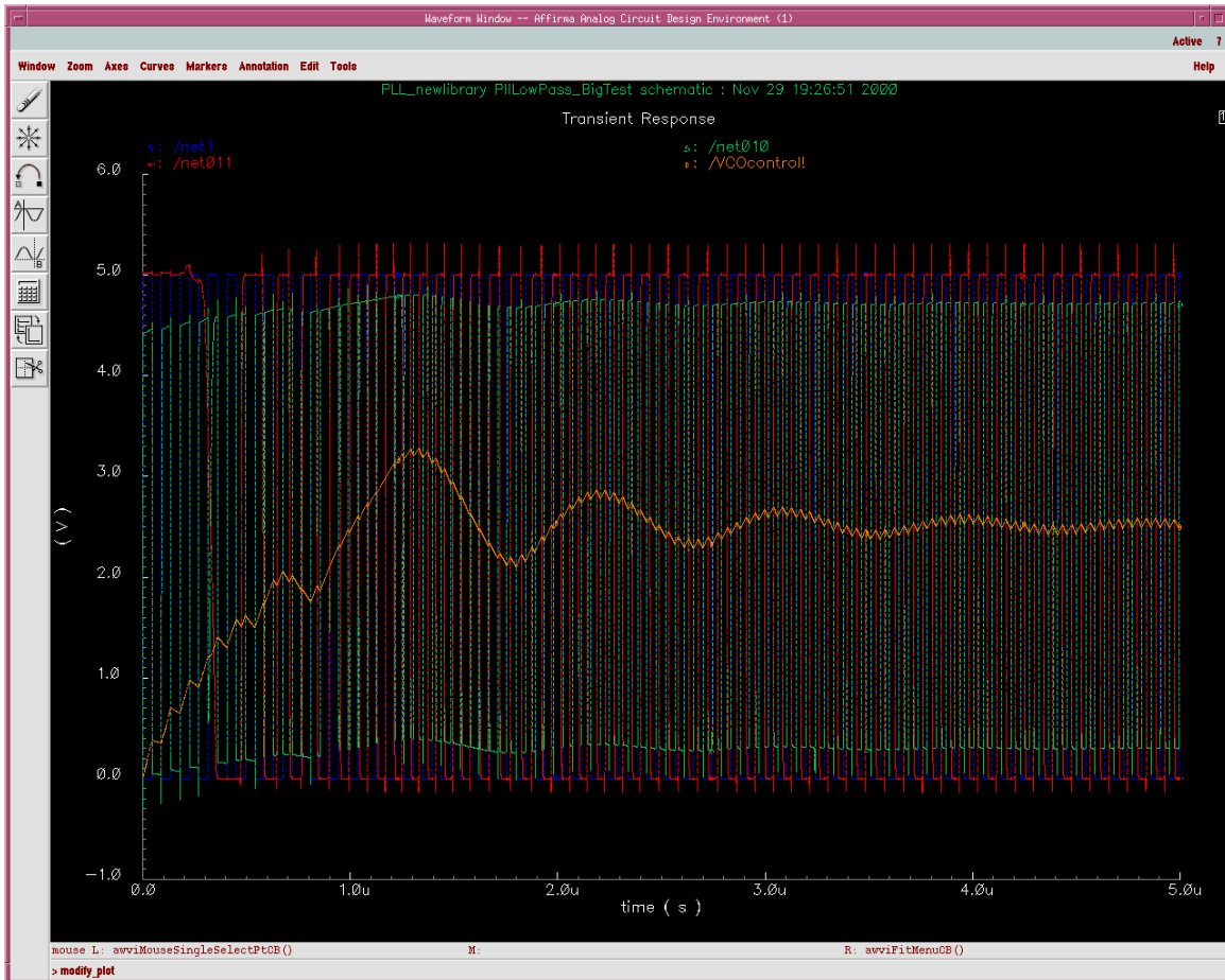
Figure 3.12 – Transient simulation of passive filter module PllLowPass_ in the PLL.
