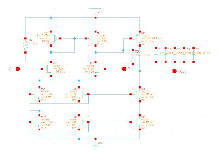
Figure 4.11: High Swing Operational Amplifier
