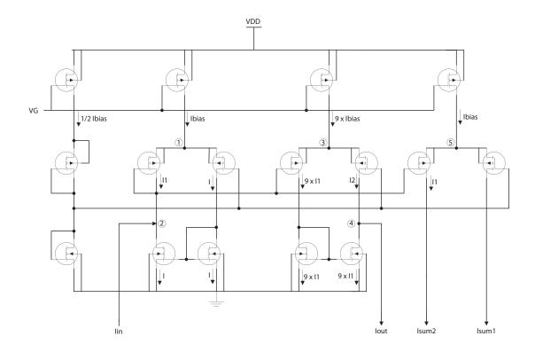
Figure 2.2: Circuit Diagram Current Limiting Amplifiers.
