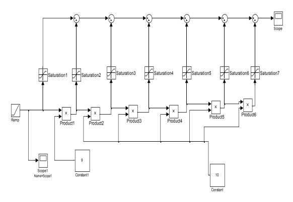
Figure 3.1: 7 stages Pseudo Logarithmic model in Simulink
