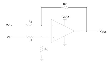
Figure 4.15: Difference Amplifier Configuration
