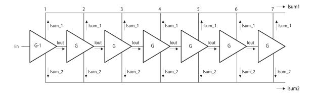
Figure 2.1: Cascaded Configuration of Current Limiting Amplifier
