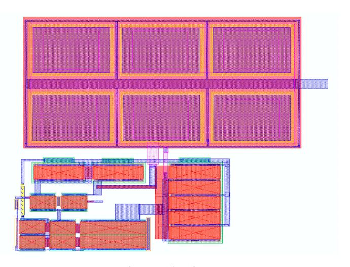
Figure 4.12: Operational Amplifier Layout
