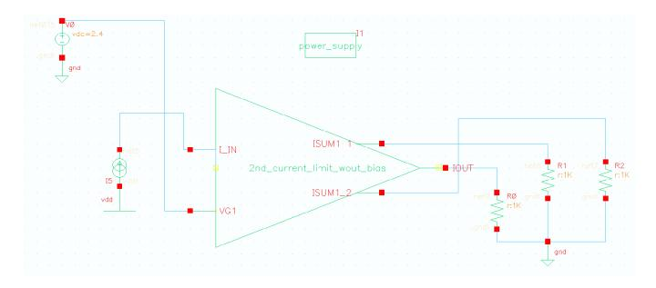
Figure 4.4: Current Limiting Amplifier Test Circuit
