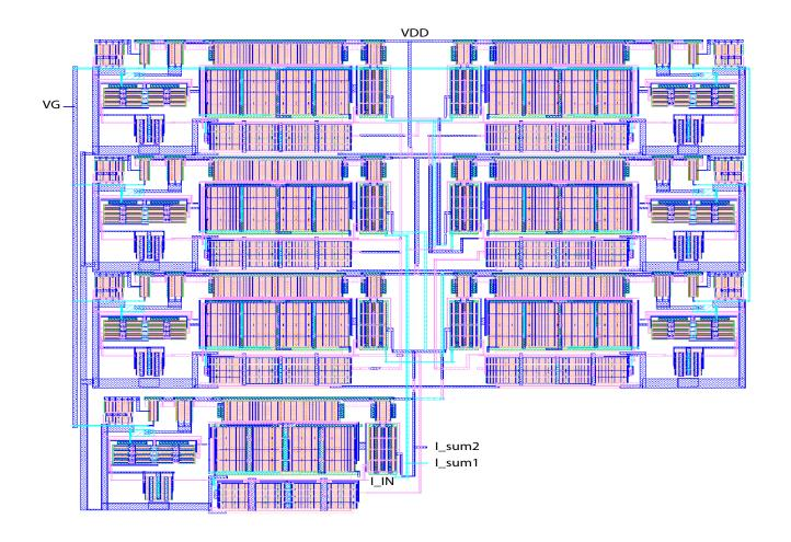
Figure 4.7: 7 Stage Current Amplifier Layout
