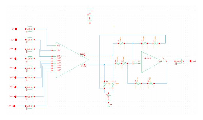
Figure 4.16: 120 dB Pseudo Logarithmic Amplifier Circuit
