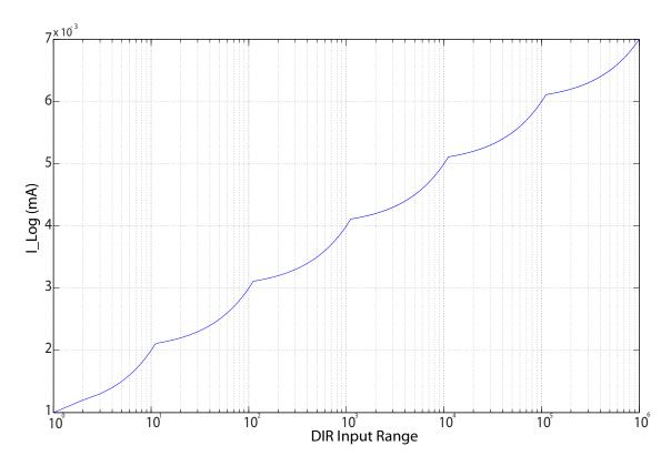
Figure 3.2: Output of the seven stage limiting amplifier
