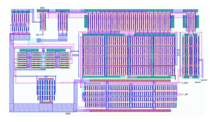
Figure 4.3: 10X Current Limiting Amplifier Layout
