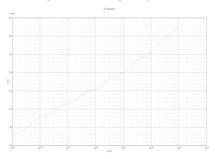
Figure 4.19: 120 dB Pseudo Logarithmic Amplifier Output Plot
