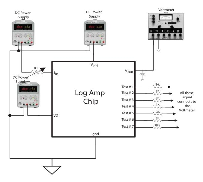
Figure 5.1: Block Diagram for Testing Log Chip
