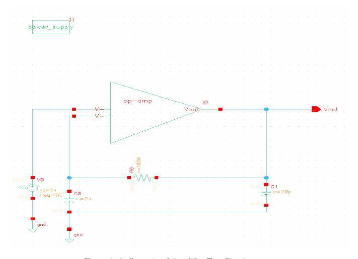
Figure 4.13: Operational Amplifier Test Circuit
