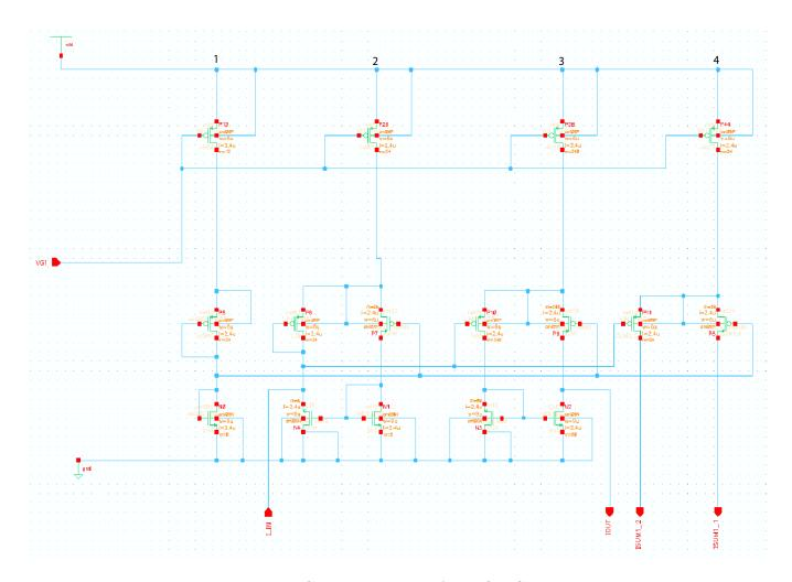
Figure 4.1: 10X Current Limiting Amplifier Circuit
