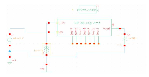
Figure 4.18: Test Circuit Pseudo-Logarithmic Amplifier
